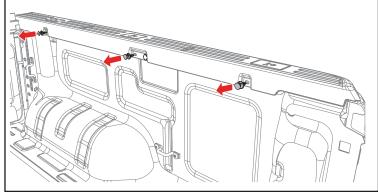
Position the cover rail (A) on the truck rail with the slotted bracket pushed all the way toward the front/cab and the bulkhead. If the truck is equipped with a drop-in bedliner, remove the foam pads located at the front of the slotted brackets.
