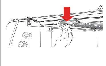
**ROLLED UP POSITION:** To drive with the cover (C) in the open position, use the cover straps (N). Roll the cover forward, twist and insert the clips into the cover clasps. Ensure that **BOTH** strap clamps are fully inserted into the clasps, pull on the end of the strap to tighten.
