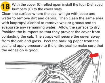
Note: If the side seals of the cover appear wrinkled, exposure to the sun will assist the seals to lay flat. Applying heat with a hair dryer or carefully with a heat gun will also smooth the seals.
