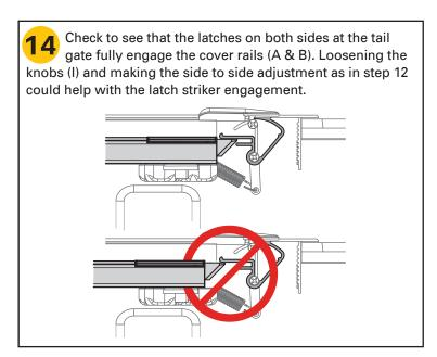
When correctly installed, the vinyl edges of the cover (C) will align squarely with the cover rails (A & B) in all four corners. The latch assembly will align with the rail locking levers at the tailgate on both sides.
