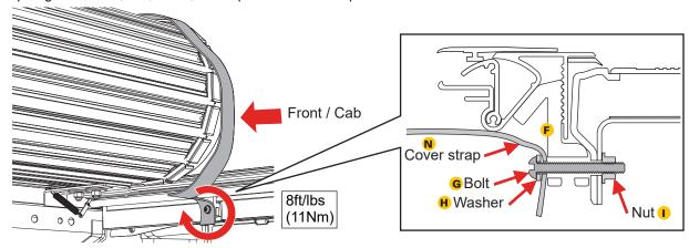
4c - FOR 2025 RANGERS: Install a rail clamp (P) at each point where the plastic clips were removed. Install the clamp up into the cover rail (A), making sure that it is inserted all the way up into the rail with the teeth of the clamp aligned with the slots in the rail. Insert a clamp bolt (G) through oversized washer (Q), through the clamp, and through the truck bed rail. Thread a clamp nut (I) onto the bolt.
