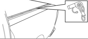
**OPENING COVER:** Pull down on the latch release cable located on either side of the cover (C) and rotate the tail rail forward and into a rolling motion. When driving with the cover open, the cover must be rolled toward the cab and secured with both strap clamps.
