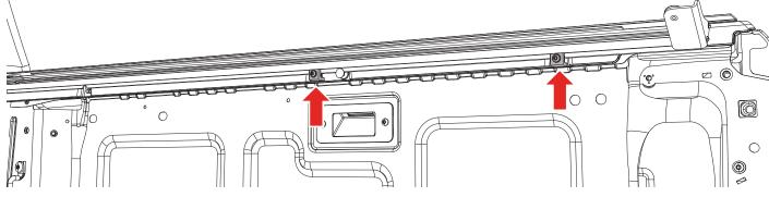
4d - FOR 2025 RANGERS: Mount the cover strap (N) and the forward most clamp (P) as shown. Use the provided oversized washer (Q) to retain the strap. Tighten to 8ft/lbs (11Nm) of torque.
