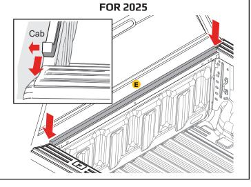
Remove three of the four factory plastic clips as shown below. Pry out the center first, then pry out the entire clip. These will not be used again unless you permanently remove the bed cover assembly.
